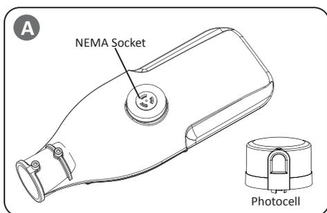
If the fixture with PHOTOCELL function, the NEMA Socket will be installed on the cover of fixture. See **A**. Fit the pins of Photocell to NEMA Socket, firmly insert and rotate Photocell to proper position.
